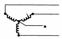
$V_L = V$  Line = Source Voltage  $V_P = V$  Phase = Phase Voltage  $V_L = V_P \times 1.732$
